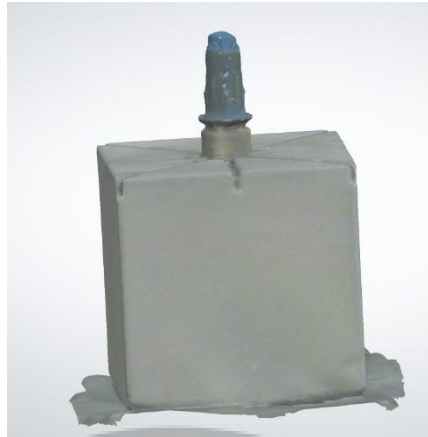
Figure 12 Ti-base abutment with PVS replica scan
