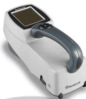
Figure 10 Colorimetric spectrophotometer, Model: Mini scan EZ 4500S, HunterLab, USA
