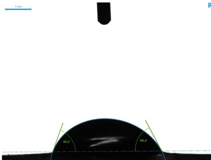
Figure 10 The contact angle of water droplets on hydrating water application substrates was assessed, with automated analysis conducted by the measuring instrument.
