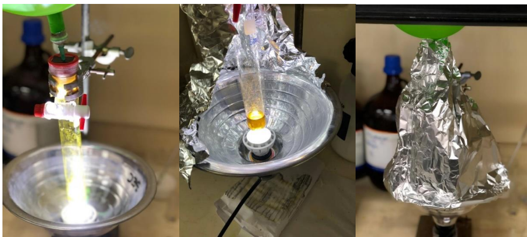
Figure 119 Set up reaction of photoredox catalysis.
