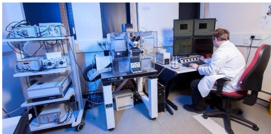
Figure 55 Leica SP5 II Confocal Laser Scanning Microscope is capable of Fluorescence Lifetime Imaging Microscopy and Fluorescence Cross Correlation Spectroscopy [111].
