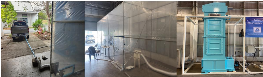
Figure 20 The developed wet scrubber tower installed in the indoor experimental room.
