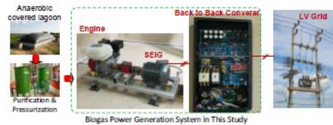
Figure 10. Prototype of the biogas power generation system.
