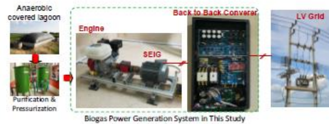
Figure 10. Prototype of the biogas power generation system.
