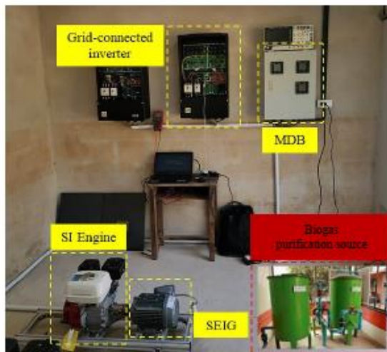
Figure 7 Experimental Setup of biogas generation unit
