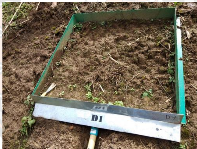
Figure 7 A micro plot structure consists of two parts; micro-plot and a pipe carrying runoff and sediments.
