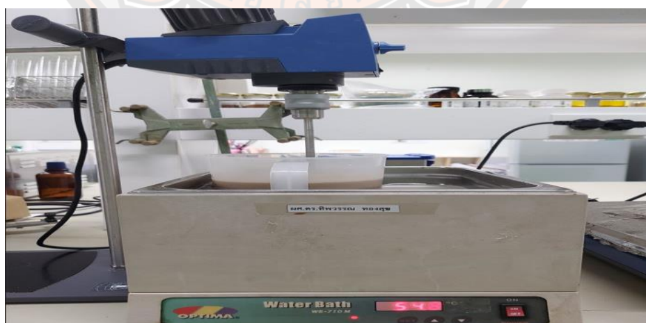
Figure 7 Hydrolysis of fermented DRB in a water bath maintained at 55°C
