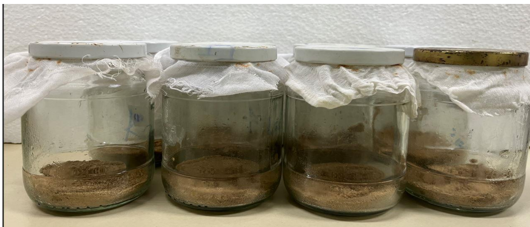
Figure 6 Solid-state fermentation of DRB at 30°C
