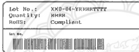
Figure 19: First label on reel: XX = Sensor Type (11 for SHT11), 04 = Chip Version (V4), Y = last digit of year, RRRR = number of sensors on reel, TTTT = Traceability Code.
