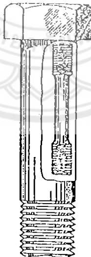
FIG. A3.5 Location of Standard Round 2-in. Gage Length Tension Test Specimen When Turned from Large Size Bolt
