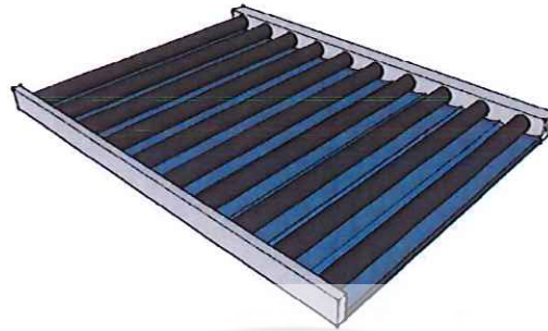
Fig.1. Evacuated tube solar collector with compound parabolic concentrators (CPC)
