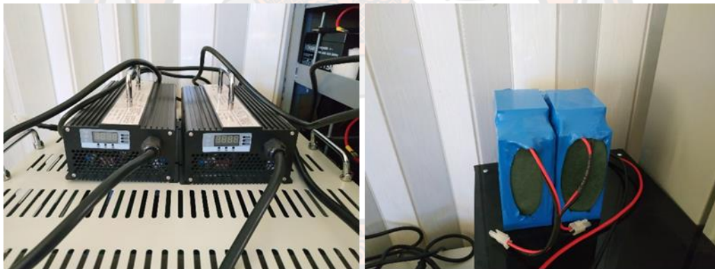
Figure 13 Battery Capacity Performance Test.
