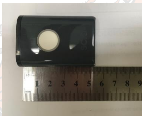
Figure 15 A picture of the SCIO spectrometer. Demonstrating of its dimensions.
