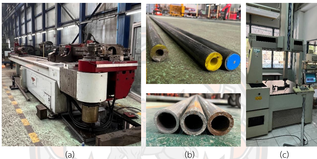
(a) Herber 76 CNC TB Bending Machine (b) Steel tube (c) CMM Mitutoyo
