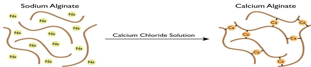
Figure 18 The ionic gelation process by the bonding of \text{Ca}^{+2} ions with polyguluronic portions of the polymer strands
