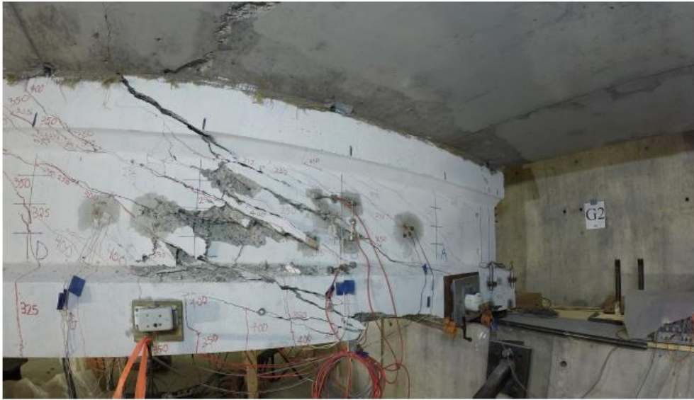
Figure 44 Web shear crushing and deck punching in G2 during LBUE looking north [35]
