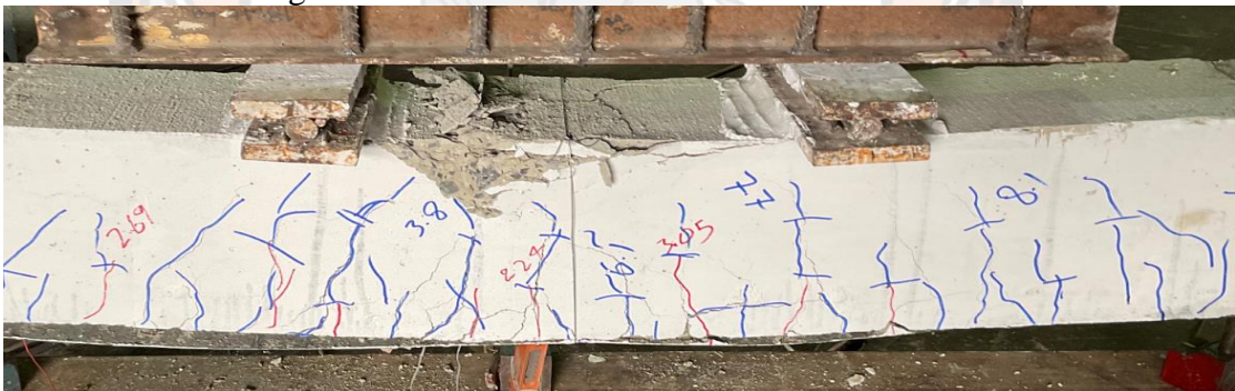
Figure 180 Failure mode of beam B05-HS50-SCA
