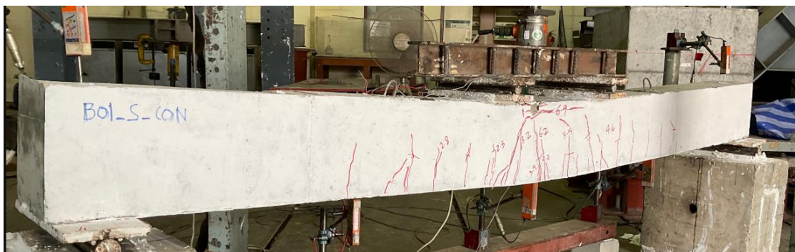
Figure 176 Failure mode of beam B01-SS-CON
