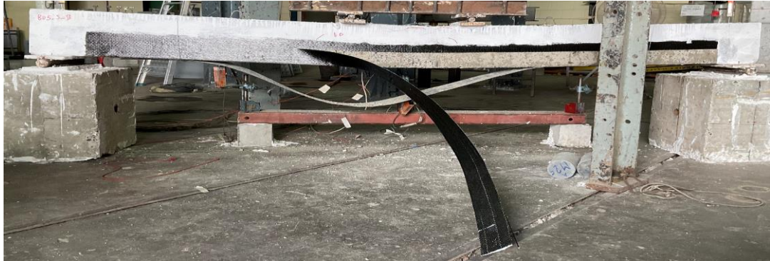
Figure 182 Typical CFRP rupture observed in 3rd group
