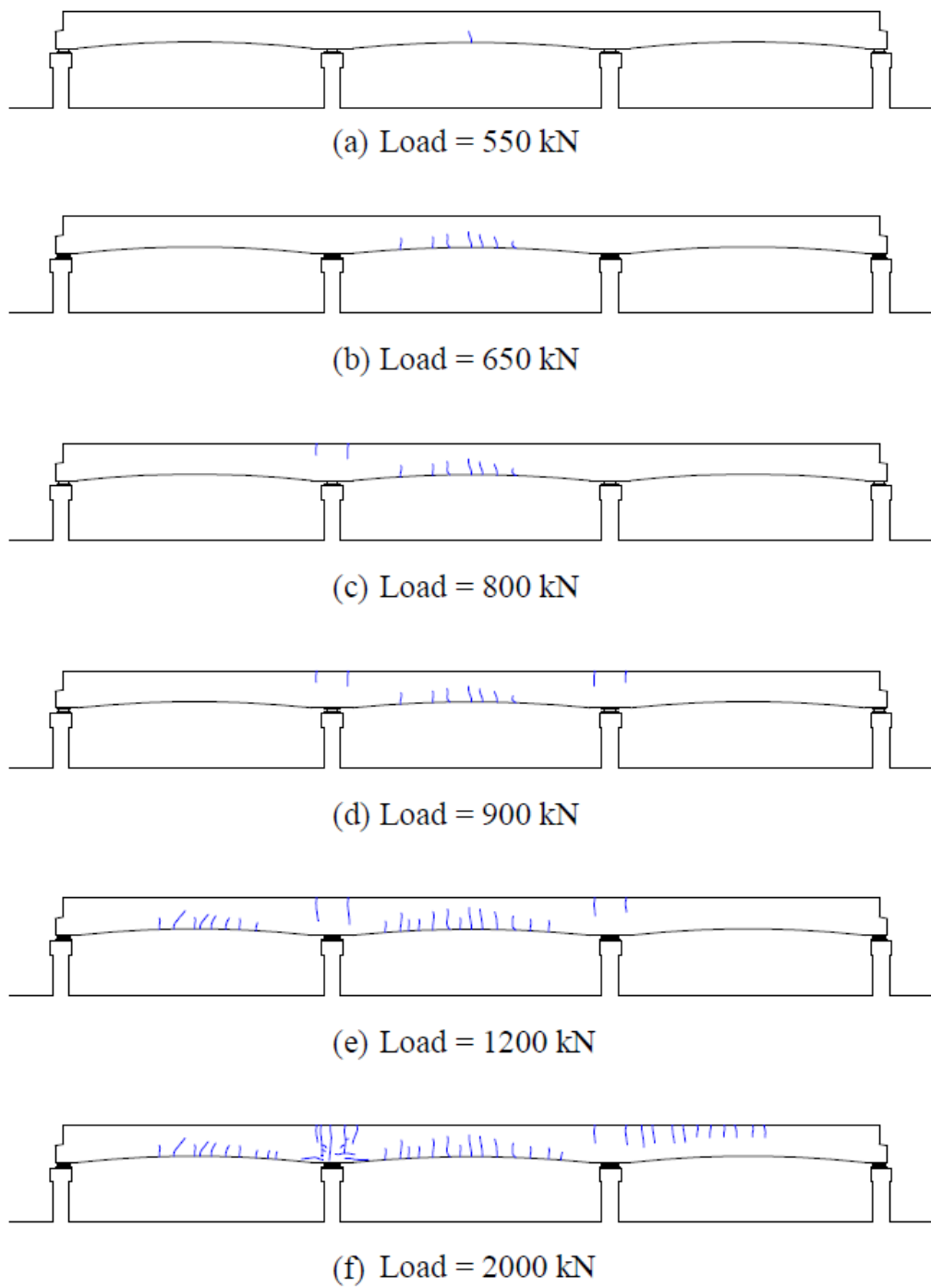
Figure 163 Cracking pattern of the FPPC girder at different loads, a) 550 kN, b) 650 kN, c) 800 kN, d) 900 kN, e) 1200 kN, and f) 2000 kN
