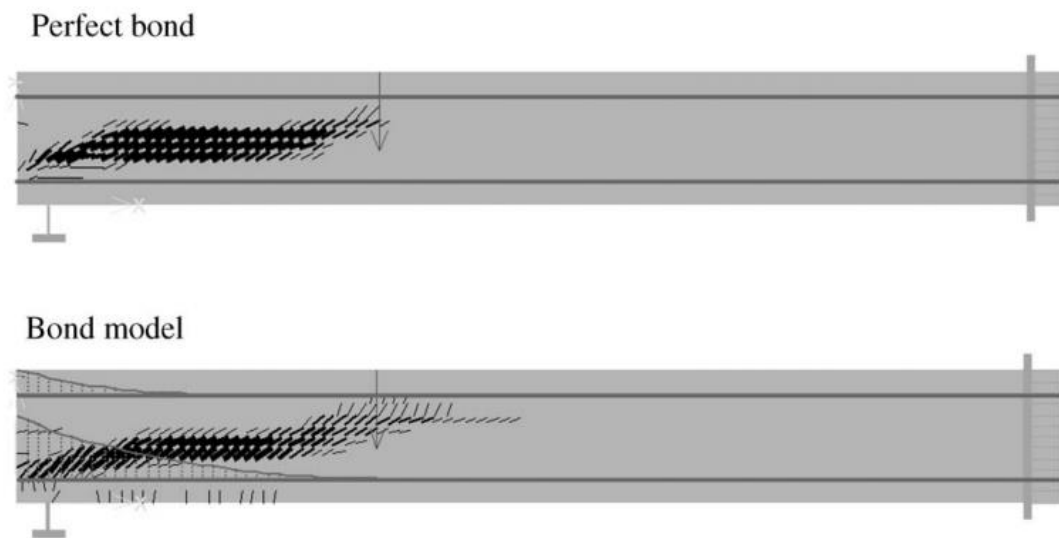
Figure 68 Cracks patterns observed in finite element analysis [40]
