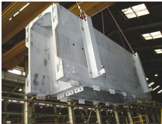
Photograph 5. rU girder segment.
