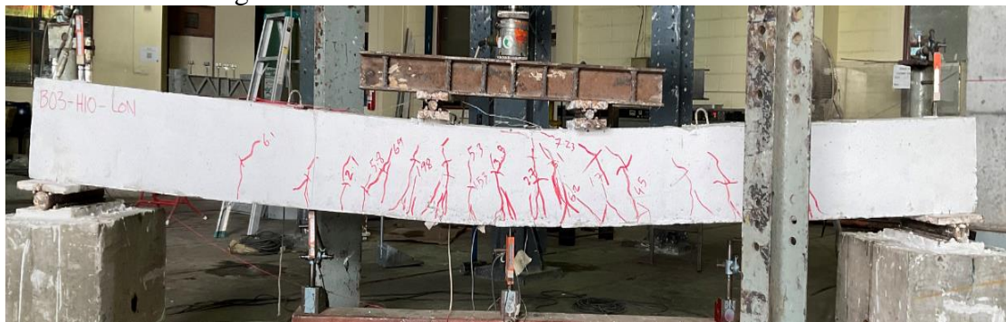
Figure 178 Failure mode of beam B03-HS100-CON
