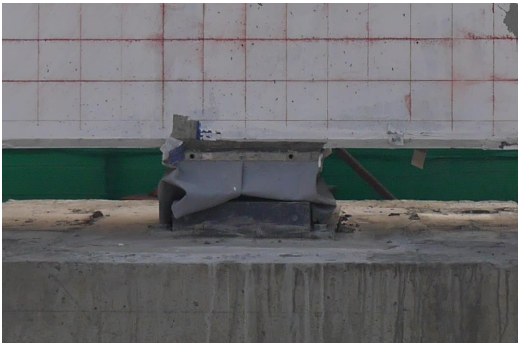
Figure 160 Bearing B-03 after test
