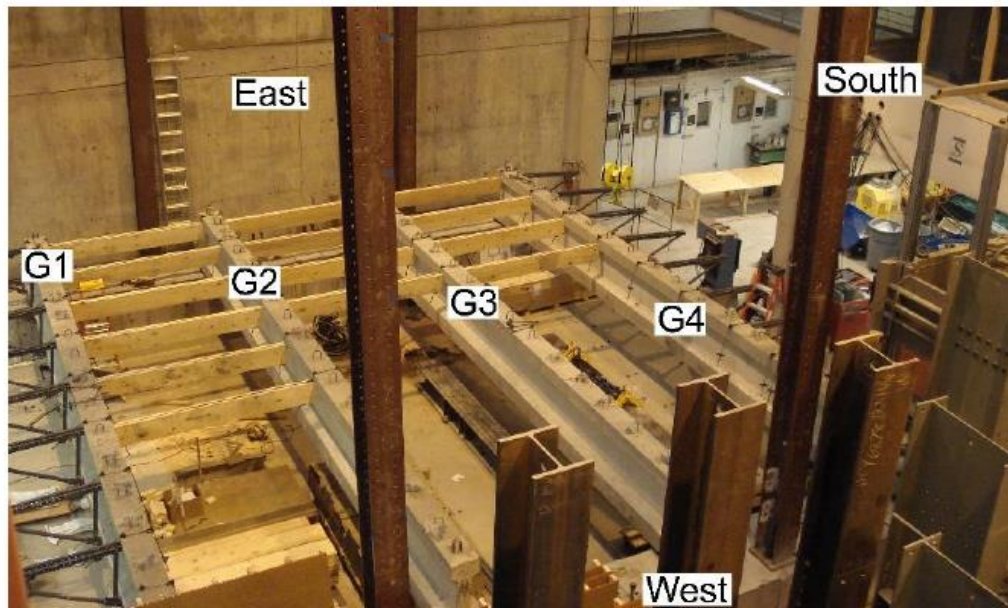
Figure 41 Laboratory bridge girder orientation [35]
