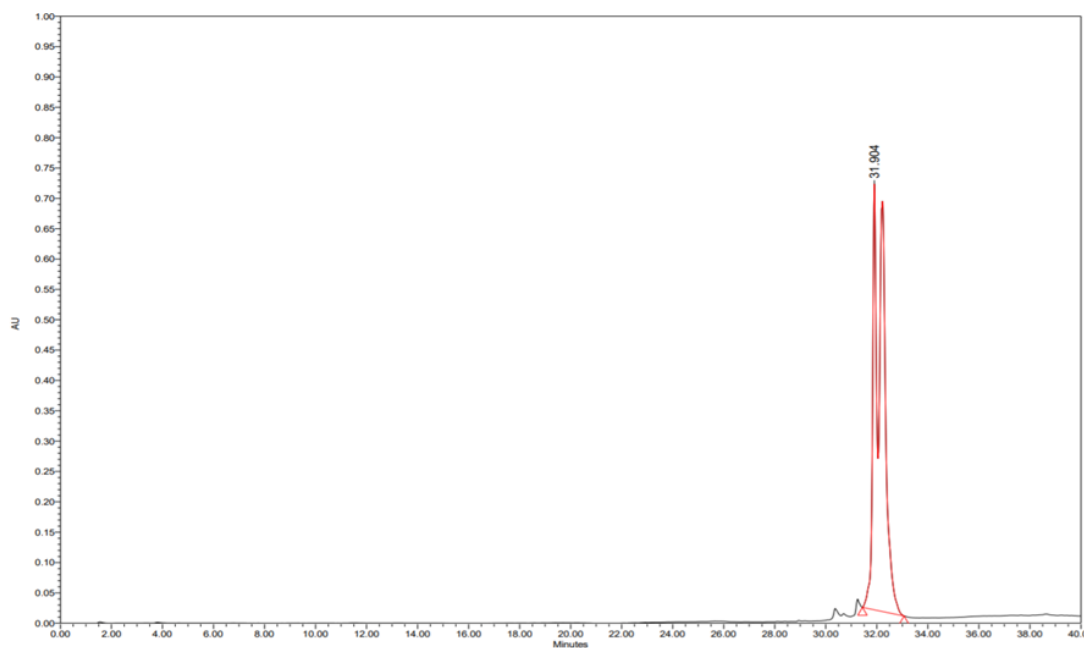
Figure 63 RP-HPLC chromatogram of PNA1. The product was observed at 31.9 min with the presence of two peaks corresponding to the 5(6)-isomers of fluorescein.
