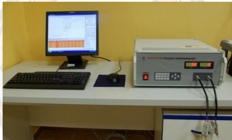
Figure 68 the computer controlled modified Sawyer Tower circuit
