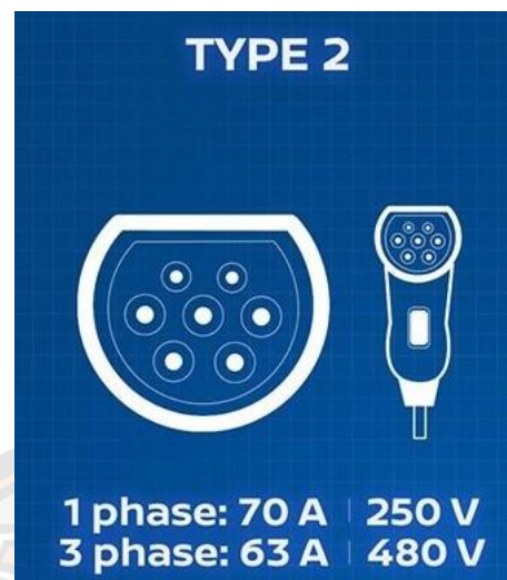
FIGURE 2 PLUG NORMAL CHARGER AC TYPE 2
