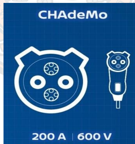
FIGURE 3 PLUG QUICK CHARGER DC CHADEMO
