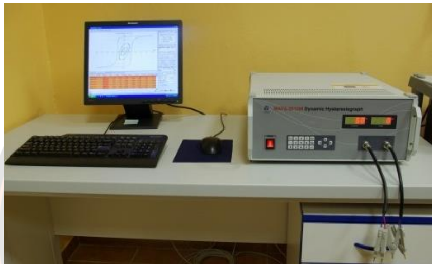
Figure 45 The computer controlled modified Sawyer Tower circuit.
