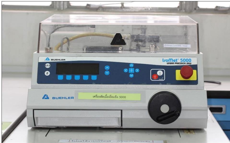
**Figure 4 The low-speed diamond saw.**
