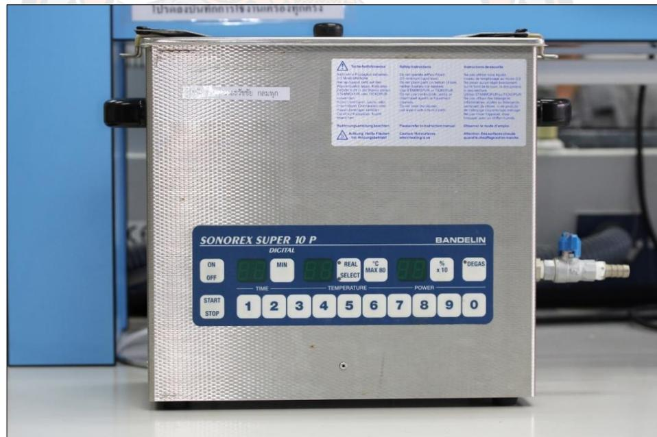
**Figure 9 An ultrasonic cleaner device.**
