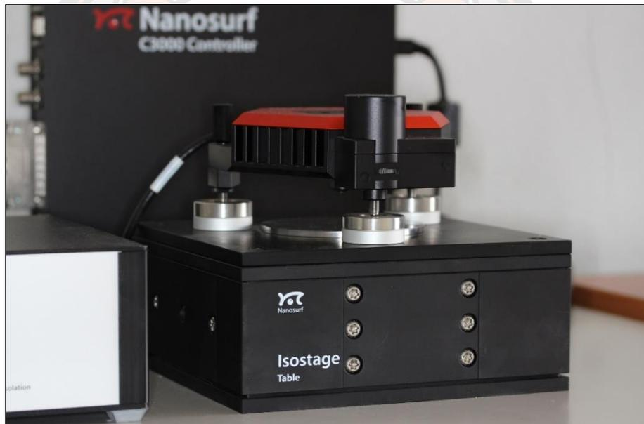
**Figure 10** An atomic force microscopy.
