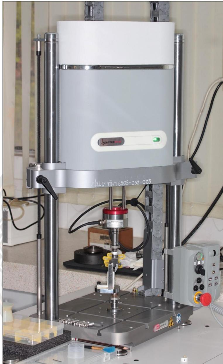
**Figure 25 The universal testing machines.**
