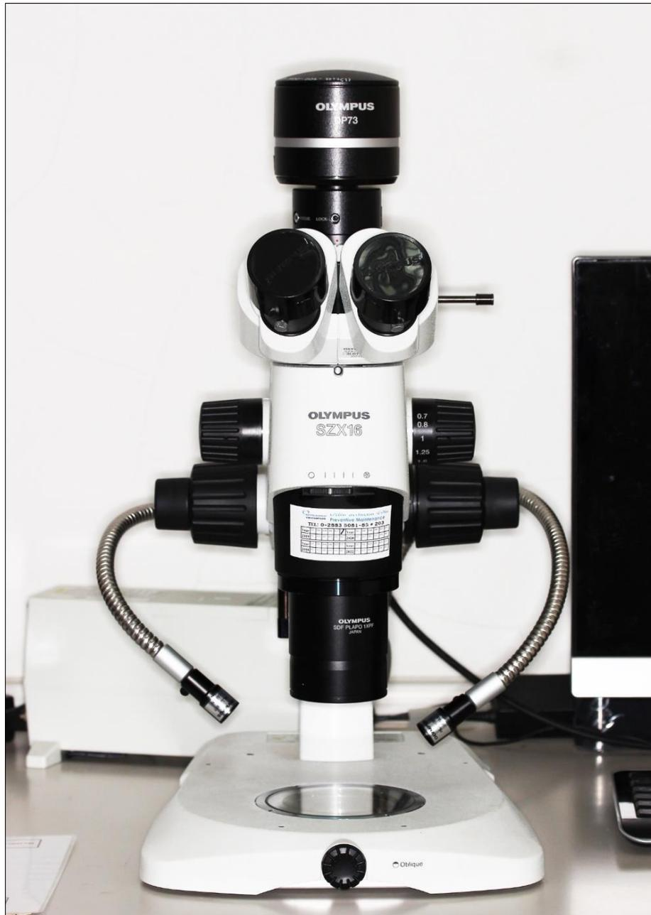
**Figure 5 The stereomicroscope.**
