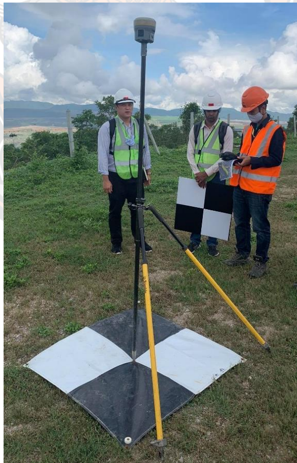
Figure 9 GNSS survey for Target as GCP in georeferencing at the study area
