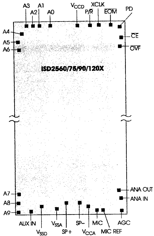
Figure 13: ISD2560/75/90/120 Products Future Bonding Physical Layout 1 (Unpackaged Die)
