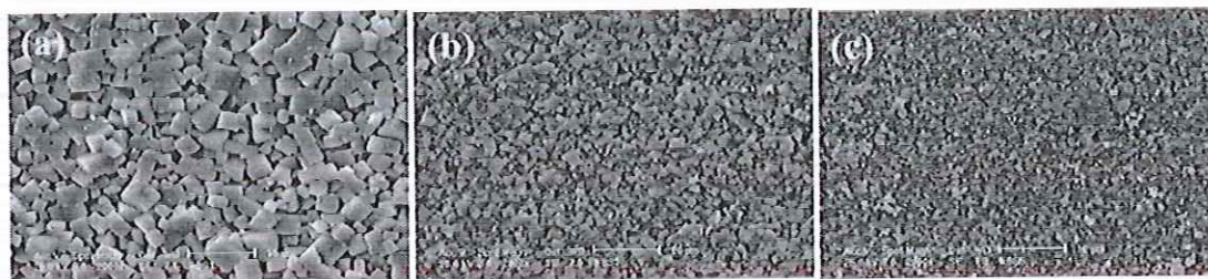
Figure 11 SEM micrographs of (1-x)\text{KNN}-x\text{BNT} ceramics sintered at 1090 \text{ }^\circ\text{C} with x equal to (a) 0.01, (b) 0.03 and (c) 0.05 [73]
