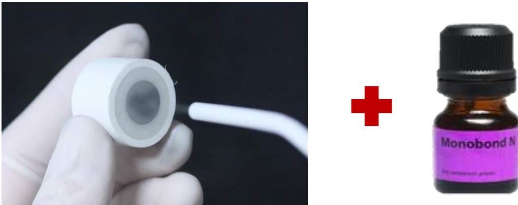
Figure 32 Sandblast of titanium disk and applied with Monobond N for Group V
