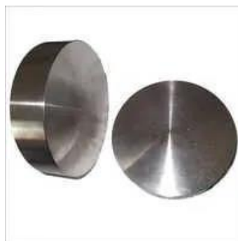
Figure 12 Titanium disk: 10 mm in diameter and 5 mm in thickness
