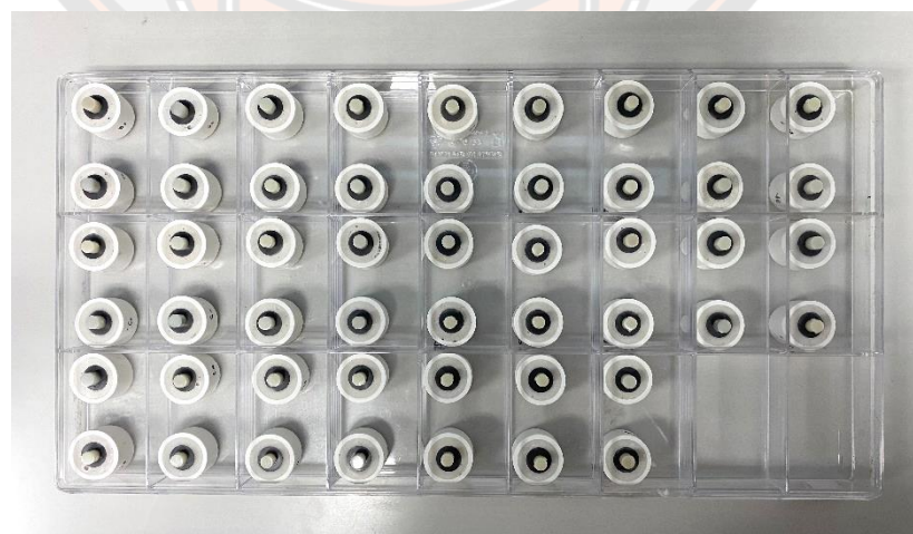
Figure 27 Stored all specimens in water for 24 hours at 37°C
