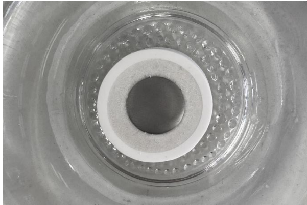
Figure 20 Treated of titanium disk with 50% H 2 O 2 15 min for Group 4
