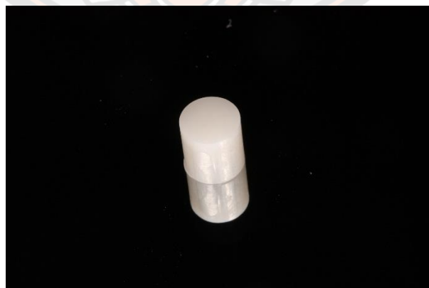
Figure 14 Zirconia disk: 5 mm in diameter and 5 mm in thickness
