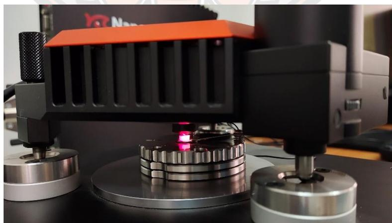
**Figure 4** The specimens' nano surface roughness evaluation by atomic force microscopy
