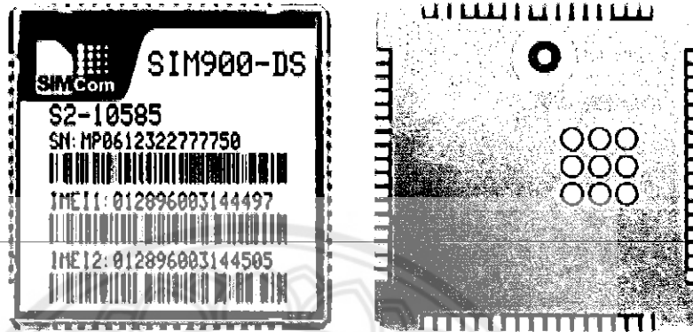
Figure 37: Top and bottom view of SIM900-DS
