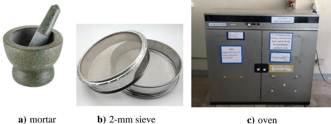
**Figure 22** The equipment for sample preparing
