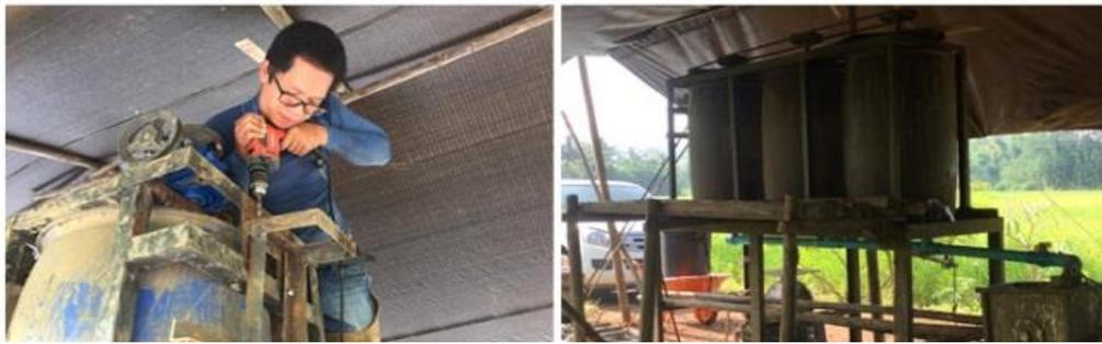
a) installed magnetic-assisted soil washing prototype and mixing tank on field
