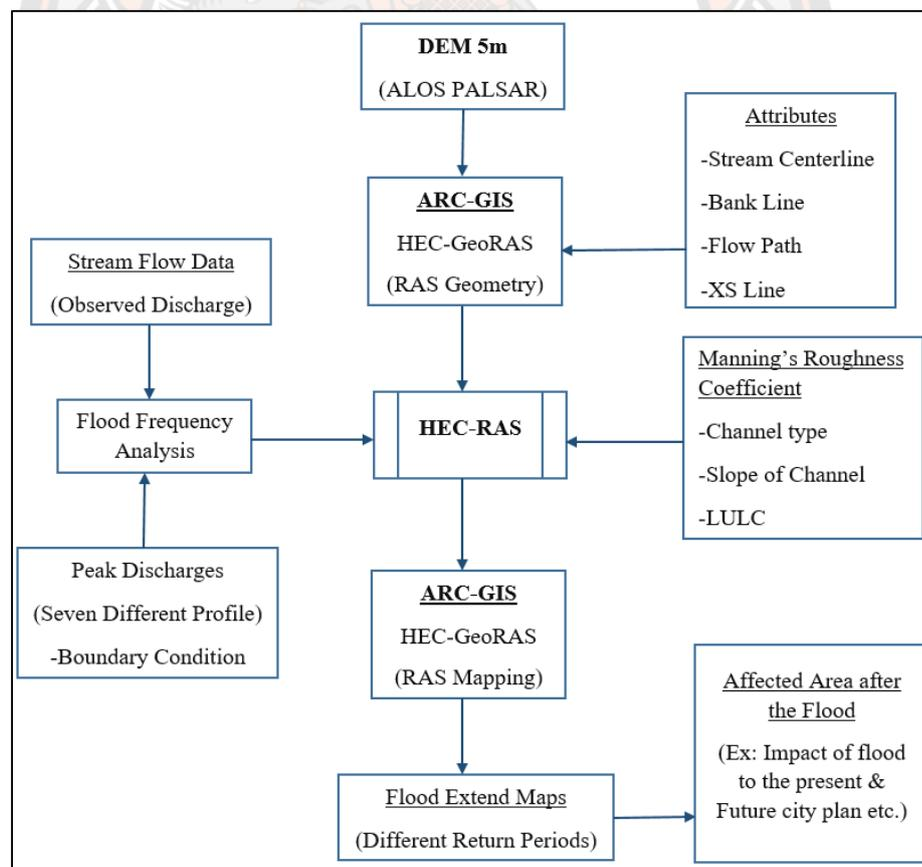
**Figure 10 Flow chart showing the modeling using ARCGIS, HEC-GeoRAS & HEC-RAS**
