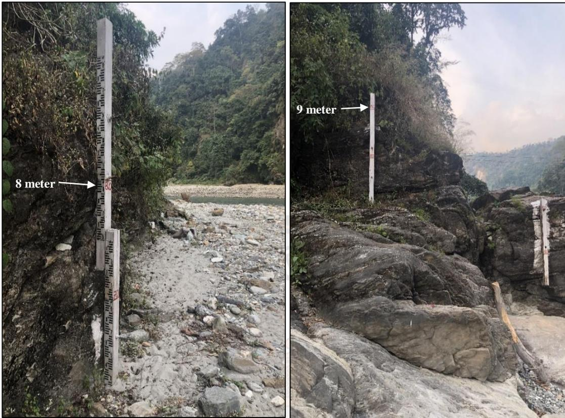
**Figure 15 Actual depth value of 2009 extreme flood event at 8m to 9m observed at Doyagang gauging station**
